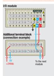
An additional terminal block can be installed on the I/O module using the two slides located in the lower part of the module case (item 11 in "General description" paragraph).
